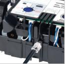
A further data cable socket has been provided for use with the secondary Digital remote control or Digital diverter. This can be accessed by carefully snapping and removing the entry pillar and connecting the cable as described above.
