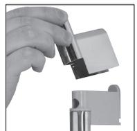
**8** If required, optional outlet flow regulators can be purchased from the Aqualisa customer helpline on 01959 560010. Fit the relevant flow regulator into the brass housing ensuring the O'ring faces the incoming flow.
