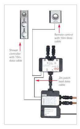
Connect the processor power lead to a double pole 3 amp fuse switched spur incorporated in the fixed wiring circuit, in accordance with current wiring rules. Ensure that this is located in an accessible, dry location and not in the bathroom.
