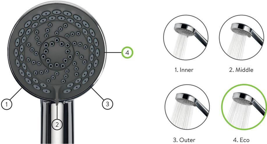
1. Rotate the spray plate lever clockwise or anti-clockwise to select the desired spray pattern. When the lever is in position 4, the water saving 'Eco' mode is selected. This provides the same spray pattern as position 3, but, depending on which water system the product is fitted to, offers up to 25% water saving.
