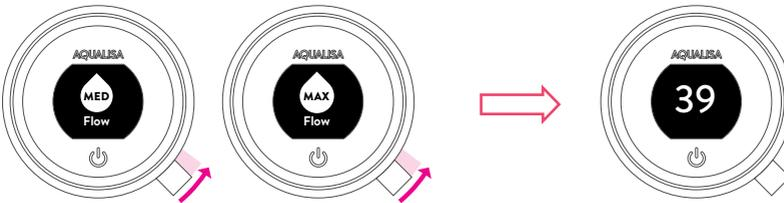
After adjusting the flow, the display will return to the temperature **Home** screen after a few seconds.
