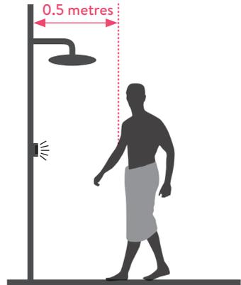
The proximity sensor detects any object directly in front, at approximately 0.5m away from the controller. See page 15 for more information.
