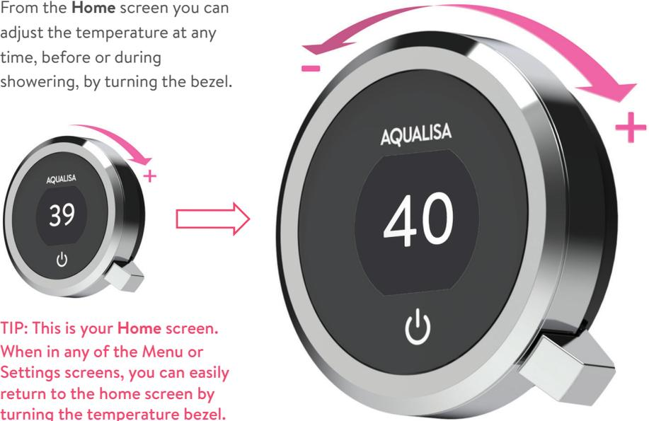
**TIP:** This is your Home screen. When in any of the Menu or Settings screens, you can easily return to the home screen by turning the temperature bezel.
