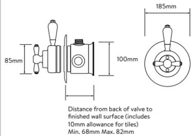
Distance from back of valve to finished wall surface (includes 10mm allowance for tiles)
