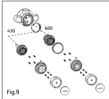
5. Remove the four screws, which secure the temperature control lever in position. Remove the lever and coloured temperature ellipses.
