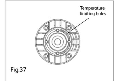
Should you wish to restrict the amount of travel of the temperature control lever to a comfort or safety zone, please refer at this point to 'Temperature Limit Pins' on page 29. If this facility is not required then please proceed as follows:
