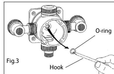
10. Work the O-ring into the seating, use a torch if necessary to check for correct location.
