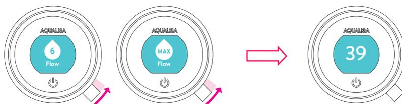
The size of the icon and the setting number will change as the flow is adjusted. After adjusting the flow, the display will return to the temperature **Home** screen after a few seconds.
