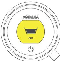
If you have a Q™ shower with a bathfill, the Q™ controller can offer specific bath functionality (storing bath depths). To enable this you must select the bath icon within this setting.
