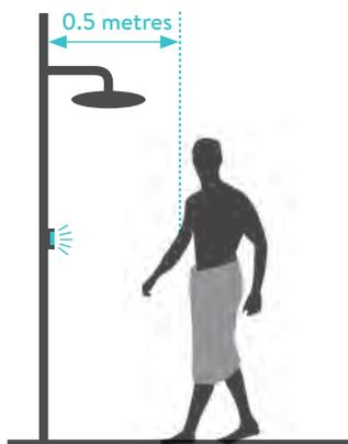
The proximity sensor detects any object directly in front, at approximately 0.5m away from the controller.
