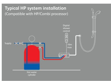
Typical thermal storage unit system installation Compatible with HP/Combi processor)
