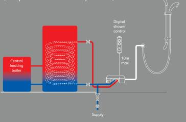
Typical combination boiler installation compatible with HP/Combi processor)
