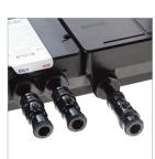
The inlet supply centres are 48mm. The inlet supply centres deviate from EN1111 and EN1287, but are deemed to be a special case. Please note arrow on isolation valve to indicate direction of flow. Compression fittings should not be used on the inlet and outlet spigots and may affect the warranty if fitted.
