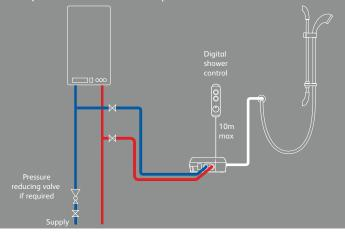
ypical pumped system installation Compatible with HP/Combi processor)
