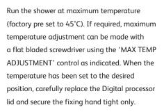
Site conditions can affect temperature settings, installer to adjust as required. ALL COPPER PIPE WORK MUST BE CROSS-BONDED AND CONNECTED TO A RELIABLE EARTHING POINT.
