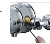
Place the assembly into the mounting ring and onto the supply pipes. Tighten the locking screw to secure the assembly to the mounting ring using the 2.5mm hexagonal key provided.
