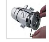
Position the mounting ring in the chase or suitable sound fixing surface. Ensure the locking screw is in the 6 o'clock position and mark the four fixing holes. Prepare the holes and secure the mounting plate to the wall using the fixings provided.
