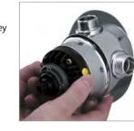
If the valve is being installed for use with a gas fired instantaneous (multipoint) water heater or a combination boiler, the cold water flow regulator must be fitted at this stage by insertion into the cold inlet connection ensuring the small 'O' ring is facing the incoming flow, prior to connection of the elbow unions.
