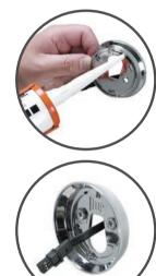
Lining up the key way, push the data cable plug into the back of the remote assembly, ensuring both rubber skirts are recessed into the connection (see diagram below), using a blunt flat bladed screwdriver or similar tool if required. To make a watertight fitting, ensure the rubbe
