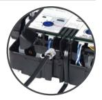
For dual outlet (divert) models the transparent end of the wired remote cable plugs directly into **port 1** of the diverter. This is indicated by the single dot. Quartz<sup>™</sup> Classic, Unity Q<sup>™</sup> and Aqualisa Smart Link<sup>™</sup> dual outlet (divert) wired remotes can only be used with dual outlet (divert) products. Please refer to the Aqualisa SmartValve<sup>™</sup> Installation Guide for further information.
