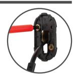
Lining up the key way, push the data cable plug into the back of the remote assembly, ensuring both rubber skirts are recessed into the connection (see diagram below), using a blunt flat bladed screwdriver or similar tool if required. To make a water tight fitting, ensure the rubber seal is no longer visible.
