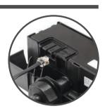
Plug in the transparent connectors of both the 10m low voltage controller and remote cables into the splitter box
