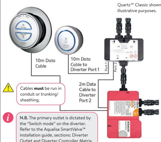
Cables **must** be run in conduit or trunking/sheathing.
